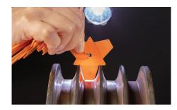
A flashlight held behind the gauge when placed in the groove, will help you observe the amount of wear
