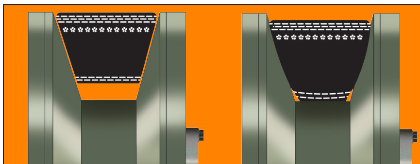
Proper Position of Belt in Sheave
