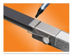
Scribe a line at the spring end of the Tension-Finder. Use this line as a reference point in case the spring slips off the belt.
