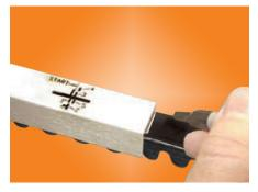
Scribe a line through the dot. The line should extend across the width of the Tension-Finder. Then go back to step 4 on page 1.
