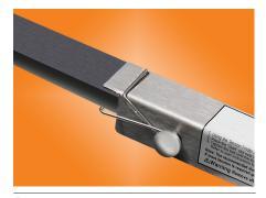
Step 5: With the line in the Start Slot attach the spring to the belt. Note: For cog belts, the best place for the spring may be in between the cogs.
