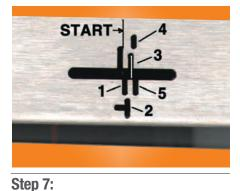
Determine the required slot for your drive from Table 1. Tighten the belt until the line has moved to the designated slot. (In this photo, the line is in Slot 3.)
