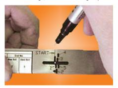
2. Put a dot at the Start Slot. Be careful not to catch the pen in the slot – you may pull the tip out of the pen.
